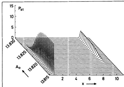
Fig. 3. Development of  $P_{st}(x)$  as a function of the injected laser amplitude  $A_0$  for  $C=20$ ,  $a=0.4$ , and  $b= 0.02317$ .
