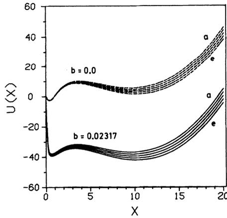
Fig. 2. These two sets of curves show the shape of the thermodynamical potential  $U(x)$  for two values of  $b$  and for the input field  $A_0$  equal to : 13.7, 13.8, 13.9, 14.0, 14.1 (a-e). The dotted lines correspond to the white-noise case given by  $b=0$ . All these curves were calculated for  $C=20$  and  $a=0.4$ .
