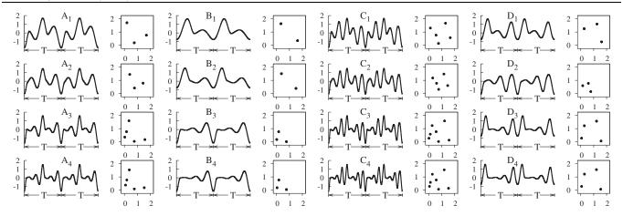
FIG. 3. Waveforms of the current x(t) along spirals A, B, C, D when moving towards the focal point  $\mathcal{F}$ . Return maps of the maxima  $x_t \times x_{t+1}$  give the number of peaks. The number of peaks of x(t) increases out of phase with respect to those of y(t) and z(t), as shown in Table I. Signals in self-symmetric spirals have much richer waveforms.
