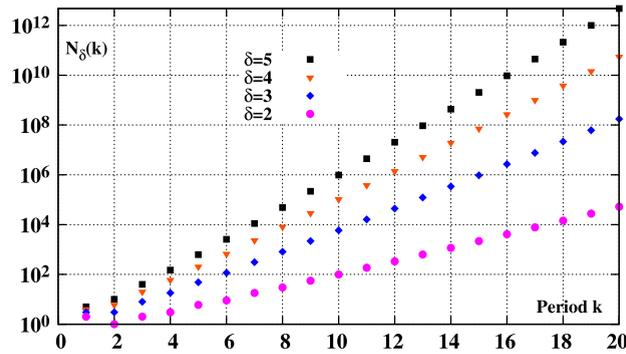
**Fig. 1.** Growth of the number  $N_\delta(k)$  of periodic orbits as a function of the period  $k$  for polynomial mappings of degree  $\delta = 2, 3, 4, 5$ , according to Eq. (5). Already for period as low as 20, cubic dynamics has about  $10^3$  times more orbits than the quadratic (logistic) map.
